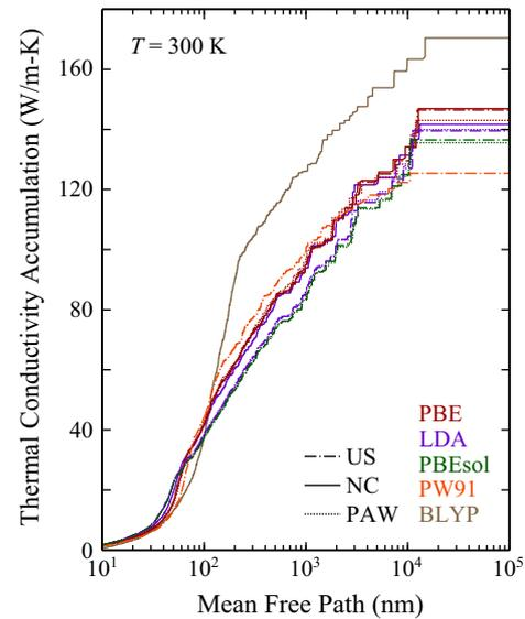
**Fig. 3.** Thermal conductivity accumulation function of silicon at a temperature of 300 K from different XC and pseudopotential types. With the exception of BLYP, all XCs result in a similar accumulation.
