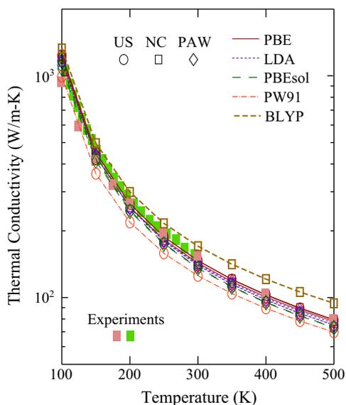
**Fig. 4.** Thermal conductivity variation of silicon with temperature from different XC and pseudopotential types. The experimentally measured thermal conductivities from Refs. [19,39] are shown as green and pink filled squares. (For interpretation of the references to colour in this figure legend, the reader is referred to the web version of this article.)
