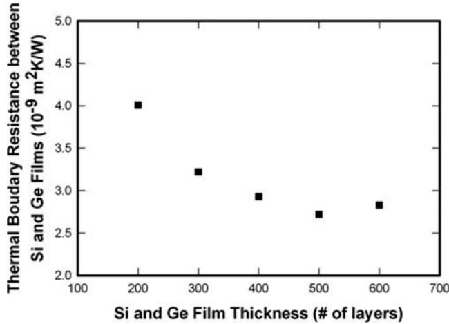
**Figure 2** Molecular dynamics simulation results of the interfacial thermal resistance between Si and Ge films as a function of the thickness of the films. The data is from Landry and McGaughey [30]. It is clear that the interfacial thermal resistance increases as the film thickness reduces, which we attribute to enhanced phonon reflection from the free boundaries as the film thicknesses gets smaller.
