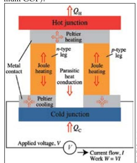
**Figure 2. Schematic diagram of a single thermoelectric refrigerator module. The hot and cold junctions are electrically insulating. This module comprises the detail that is the oval marked "Refrigerator" in Figure 1(a).**
