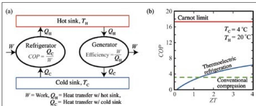
**Figure 1. (a) Thermodynamic cycles for refrigeration and power generation. In a thermoelectric refrigerator, work input as electrical power allows for heat removal from a cold sink. In a thermoelectric generator, heat transfer from a hot sink produces an electrical potential. (b) Coefficient of performance for a refrigerator operating at room temperature.**
