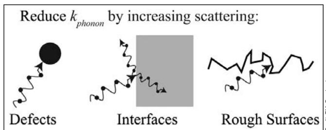
**Figure 3. The phonon contribution to thermal conductivity can be reduced by adding defects, interfaces and free surfaces that can scatter phonons. Limits to thermal conductivity are now being reached, but there is still potential to increase the Seebeck coefficient by manipulating the electronic band structure.**
