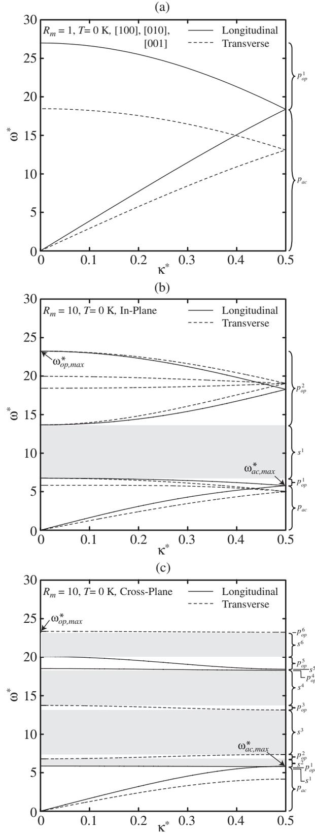
FIG. 3: (a) Phonon dispersion curves for the monatomic crystal. The dispersion characteristics are the same in the [100], [010], and [001] directions. All branches correspond to acoustic phonons, and have been folded over at  $\kappa^* = 0.5$ . Phonon dispersion curves for  $R_m = 10$ : (b) in-plane and (c) cross-plane directions. The maximum acoustic and optical frequencies are noted, and the stop bands are shaded.
