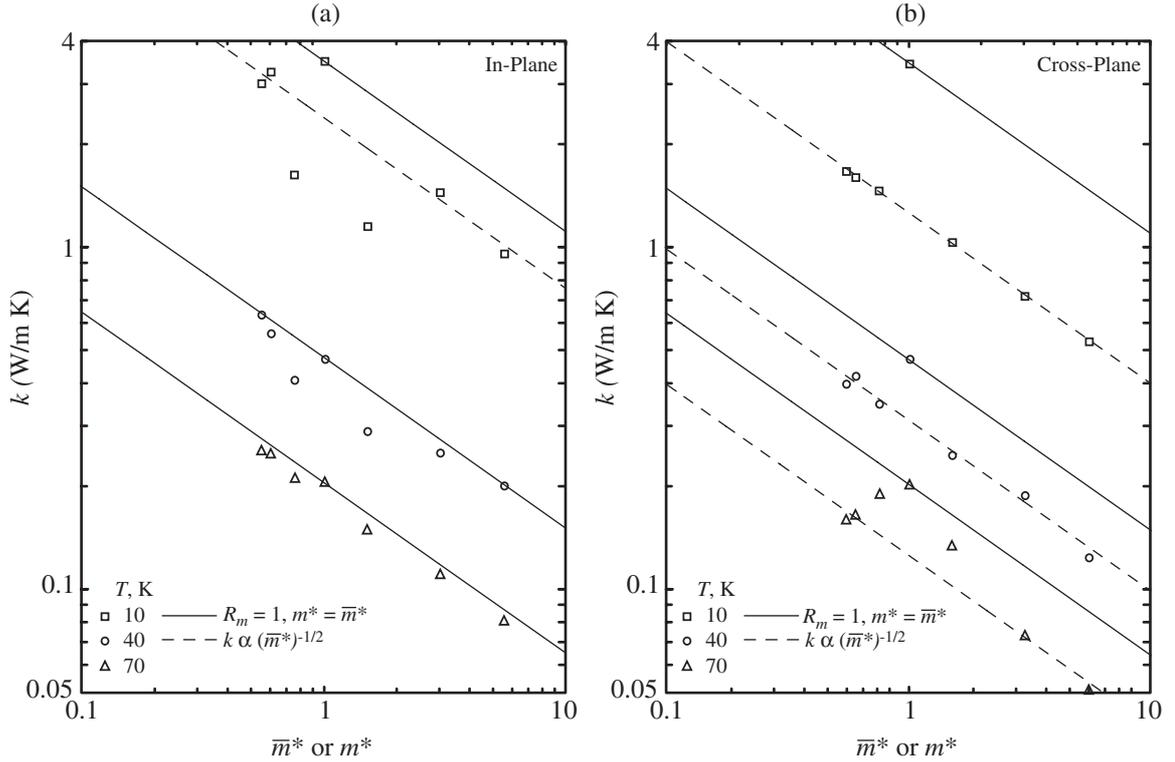
FIG. 8: Thermal conductivity at temperatures of 10 K, 40 K, and 70 K in the (a) in-plane and (b) cross-plane directions plotted as a function of the average atomic mass in the system. Also plotted is the thermal conductivity of the equivalent monatomic systems where each atom has a mass  $\bar{m}^*$  (solid line). The dashed lines correspond to  $k \propto (\bar{m}^*)^{-1/2}$ , and are fit to the data by visual inspection.
