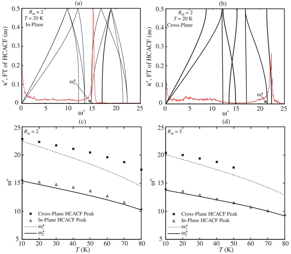
FIG. 9: (Color online) (a) In-plane and (b) cross-plane dispersion curves (black lines) superimposed on the respective HCACF spectra [red (gray) lines] for  $R_m = 2$ ,  $T = 20$  K. Comparison of the peaks in the HCACF to the associated frequencies in the quasi-harmonic dispersion curves for (c)  $R_m = 2$  and (d)  $R_m = 5$  in the in-plane and cross-plane directions, plotted as a function of temperature.
