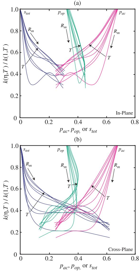
FIG. 10: (Color online) Thermal conductivity at all temperatures and mass ratios considered, scaled by the appropriate  $R_m = 1$  value, plotted against the phonon dispersion metrics  $p_{ac}$  [pink (light gray) lines],  $p_{op}$  [green (medium gray) lines], and  $s_{tot}$  [blue (dark gray) lines]. To best see the trends, smooth curves through each of the data sets are plotted.
