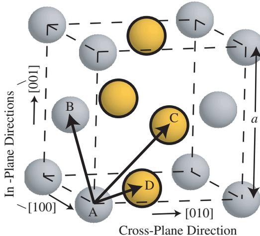
FIG. 2: (Color online) The four-atom unit-cell of the layered diatomic crystal. If the four atoms are equivalent, the crystal structure is face centered cubic. If A and B have a different mass than C and D, the crystal structure is simple cubic. The arrangement chosen leads to planes with a thickness of one atomic layer stacked in the  $[010]$  (cross-plane) direction.
